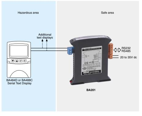
The BA201 communications isolator is a dedicated interface for connecting intrinsically safe BEKA Serial Text Displays to a safe area computer system. The isolator provides intrinsically safe galvanic isolation between the safe and hazardous areas, plus conversion of the RS232 or RS485 safe area serial data to the dedicated communications signalling required by BEKA Serial Text Displays.
